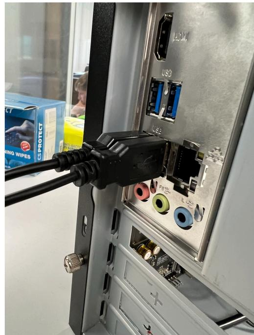
Figure 4: The USB plugged into the correct port.
