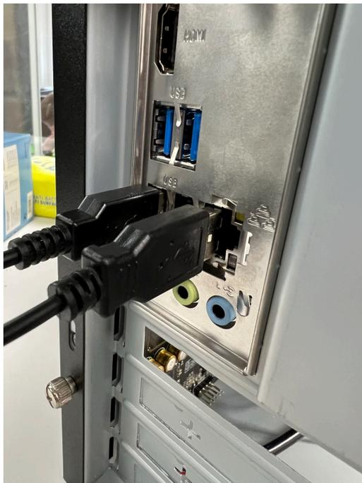
Figure 3: The USB is plugged into an RJ45 port.
