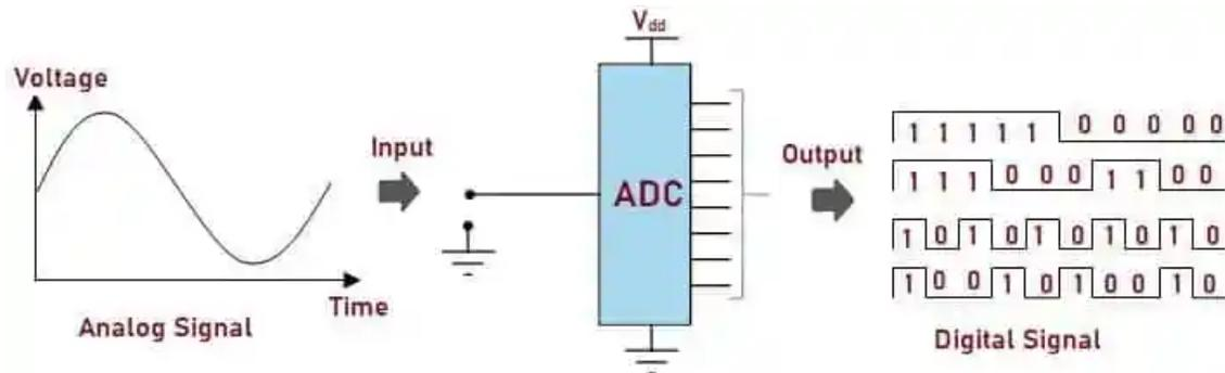
Figure 5: Basic example of how an analogue signal is converted to be digital
