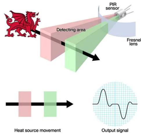
Figure 8: Example of a PIR sensor
