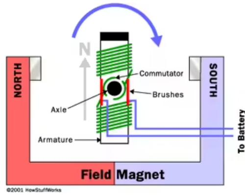
Figure 9: Example of a DC motor
