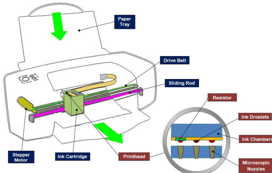
Figure 11: Internals of an Inkjet printer
