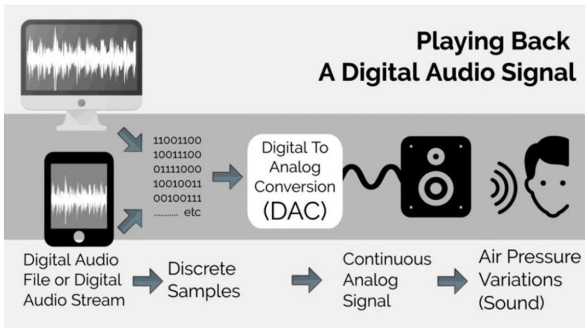
Figure 4: Basic example of how digital audio is played on an analogue speaker
