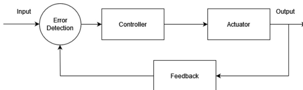
Figure 14: Flowchart of a Closed Loop System
