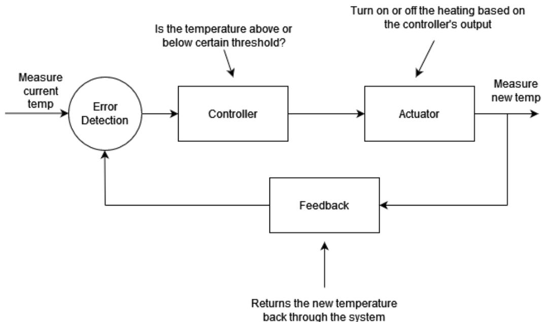
Figure 15: Flowchart of a Central Heating Proportional Control System
