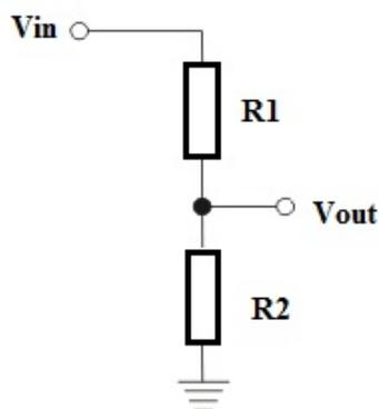
Figure 7: Resistive-Type Voltage Sensor
