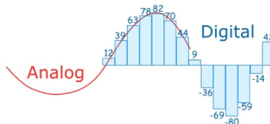
Figure 3: Basic example of an analogue signal being quantised into a digital signal
