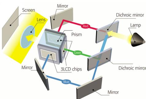
Figure 10: Internals of an LCD projector
