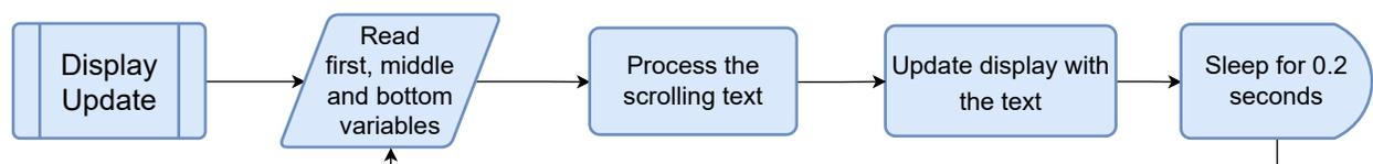
Figure 5: Flowchart of Beam Sec's display update function
